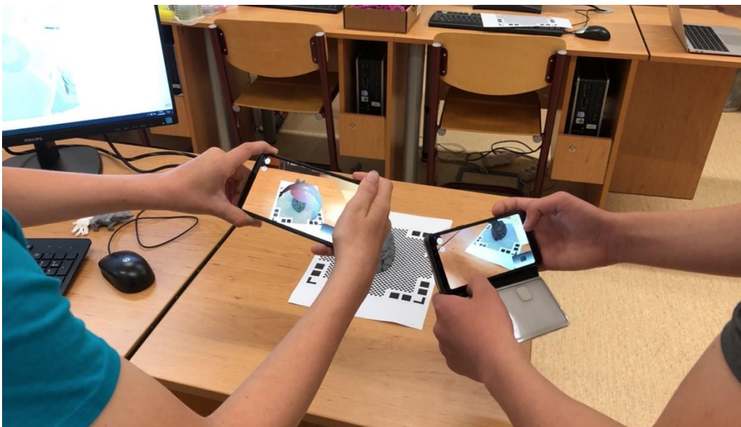
Picture 12: 3D scanning via mobile phone
